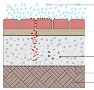
Sedement and oil on surface Sedement trapped in laying course and upper geotextil (if present)
